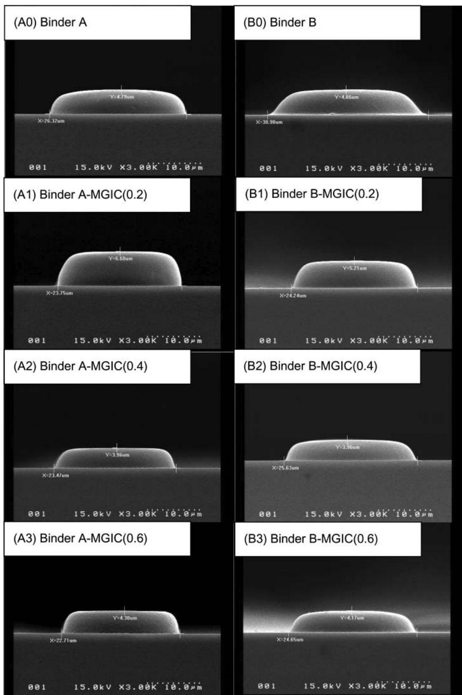
Figure 10. SEM diagrams of photoresist of runs A0–A6 and B0–B6. ( Continued )
